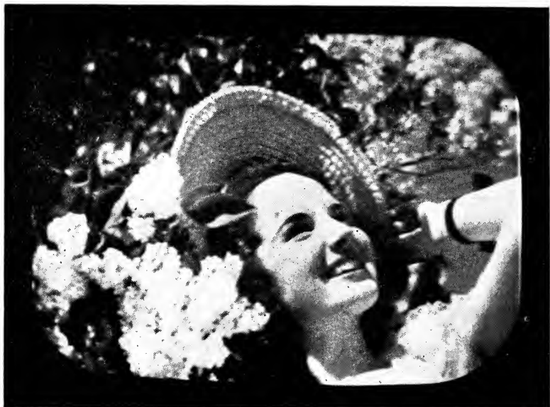
Fig. 6. Picture transmitted with 4.5-mc cutoff frequency, uncrispended.
